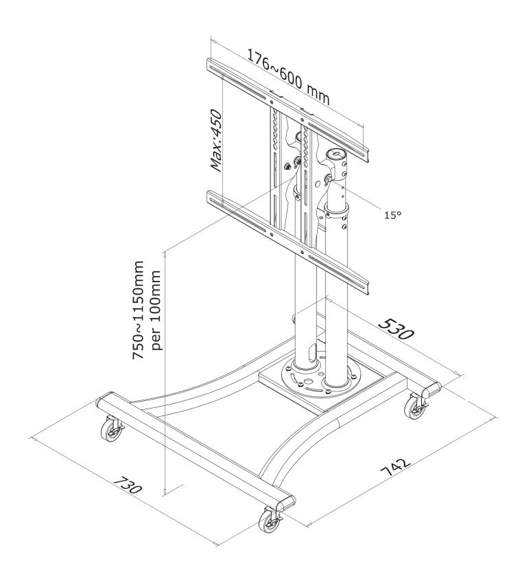
Neomounts Measuring unit: mm
